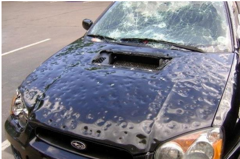
Large-hail damages on a car
