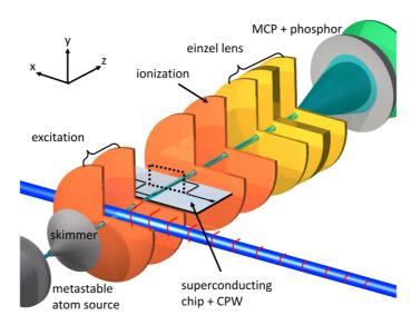
Sketch of the main experimental setup: helium atoms propagate through the cryogenic setup along the z axis. They are excited to a Rydberg level by a combination of optical and microwave pulses. They interact with a sample (2D or 3D cavity) and are ionized. The resulting electrons are detected on a micro-channel plate (MCP).
